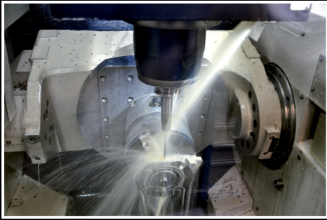
The WDO-10D in action drilling at a hole depth of 58 mm in super duplex stainless steel with a 410 HB hardness.
