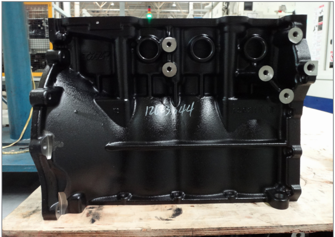
A cylinder block made of HT250 (equivalent to gray cast iron) with a 180~220 hardness.
